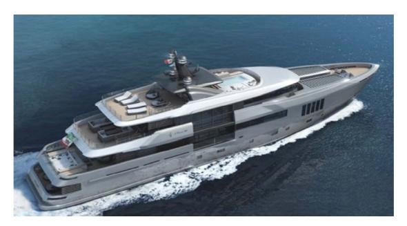
With exterior design by Jure Bukavec of Unielle Design, the C-Force 50 will feature a steel hull and aluminum superstructure. She will have a top speed of 17.3 knots and a cruising speed of 16.3 knots.
